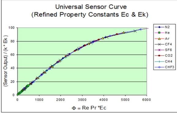
Figure 4: Each sensor is N2 calibrated and a universal sensor calibration curve as well as Similarity Theory is used to determine the MultiFlo process-gas calibration curve (US Pat #7,043,374)
