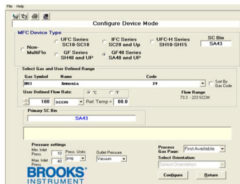
Figure 11: The process gas and flow range can both be changed from this screen, as well as the reference temperature and the MFC's pressure settings.
