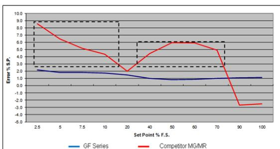
Figure 7: Multi-Gas/Multi-Range performance (N2 calibration, SF6 accuracy)
