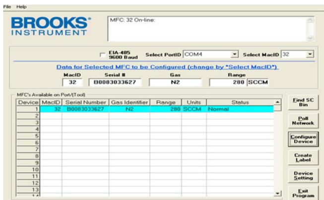
Figure 10: MultiFlo Configurator after network has been polled and connected device located.
