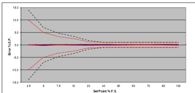
Figure 6: Brooks GF Series and Competitor perform comparably within specification on Nitrogen
